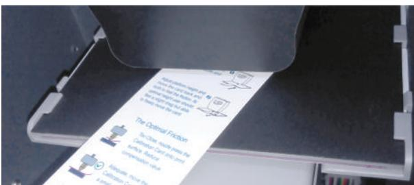
4\ Raise the platform until it is just touching the nozzle. Move the Calibration Card between the nozzle and the platform to see if there is any resistance.
