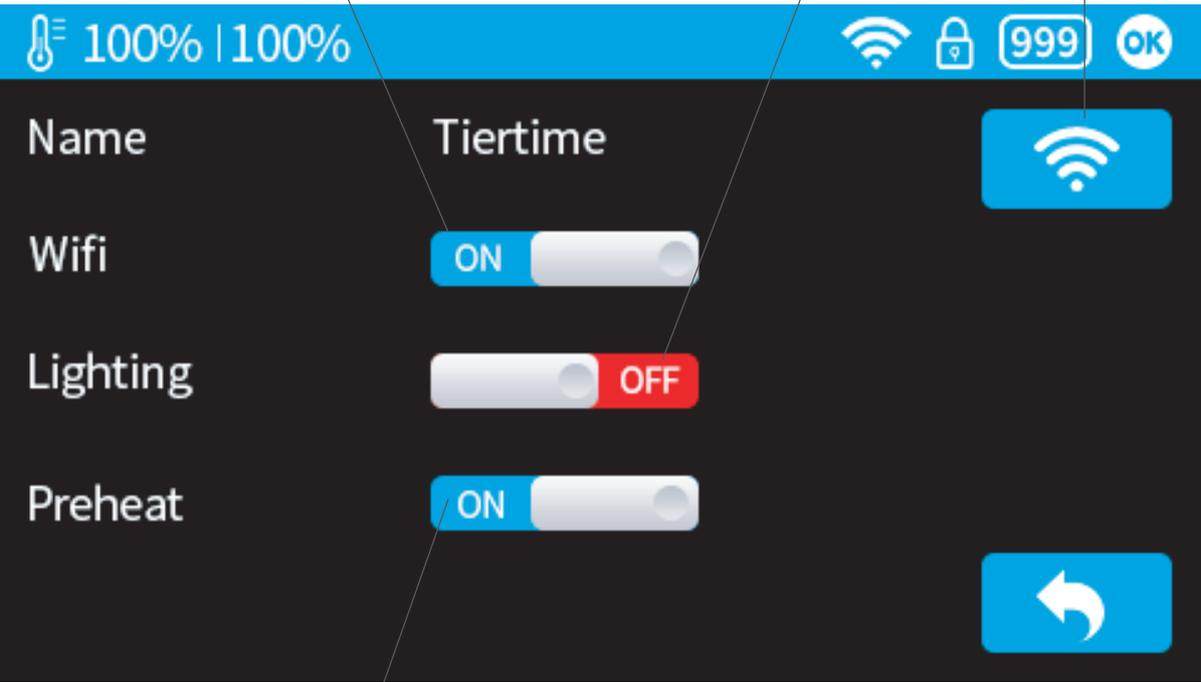
Preheat switch, when turned on, for every print job, the printer will first preheat 15min before proceed to printing.
