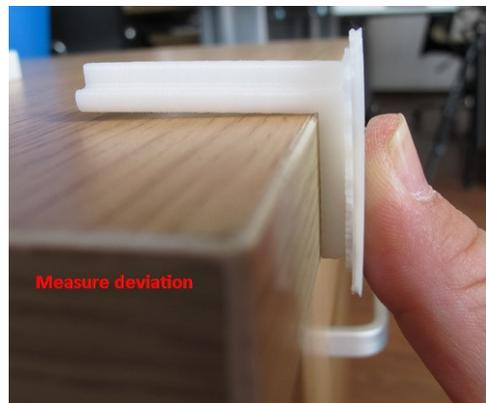
**IMPORTANT NOTE:** Before you enter any new calibration values, always click the “Reset” button, otherwise the new values get added to the old ones. Before you enter any new values, the bar at the very top of the screen should read: XY: 0.00 deg / XZ: 0.00 deg.
