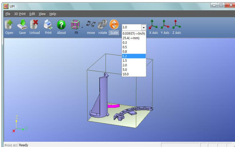
**Unit Conversion:** This option is provided as a convenient way to convert metric models to imperial, and vice versa. To convert an imperial model to metric, select the 25.4 option from the scale menu and click “Scale” again. To convert from metric to imperial, select the 0.03937 option and click “Scale”.
