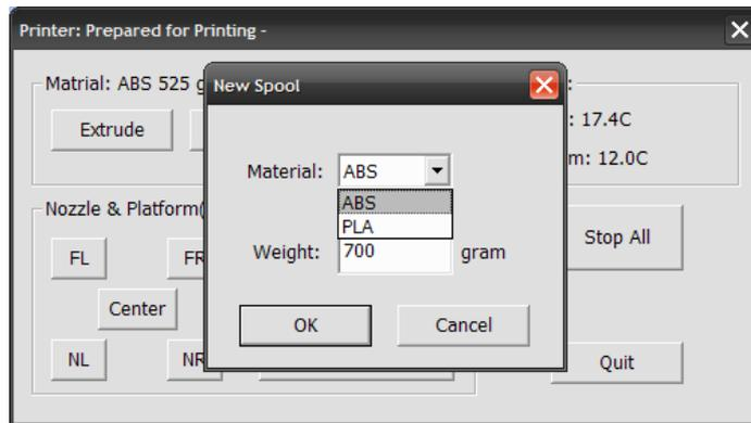
**TIP:** An empty spool weighs about 280 grams so, if you are installing a partially used spool, weigh it, and subtract 280 grams from the weight. This gives you the value to enter into the material text box.
