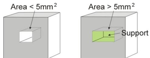
**Support - Area:** The surface area above which support material gets used. When you choose  $5\text{mm}^2$ , for example, there will be no support if the overhanging area is less than  $5\text{mm}^2$ .
