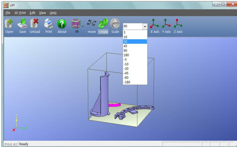
**Scaling the model:** Click “Scale”, choose or input a scaling factor in the text box, and then either scale the model uniformly by clicking the scale button again, or choose the axis around which you want to scale if you only want to scale in one direction.
